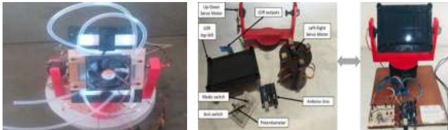
Fig.7.2 Solar panel cooling composition of solar tracker
